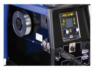
The SP-2 has 2 dedicated wire spools (Aluminum, Silicon Bronze or Steel) and 2 torches. Change between Silicon Bronze or Steel by changing the wire spool. The software is smart, just grab the desired torch click the trigger once and the software changes to the correct weld settings and gas automatically.
